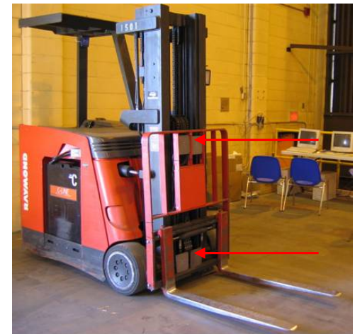
Fork-lift Mounted RFID
