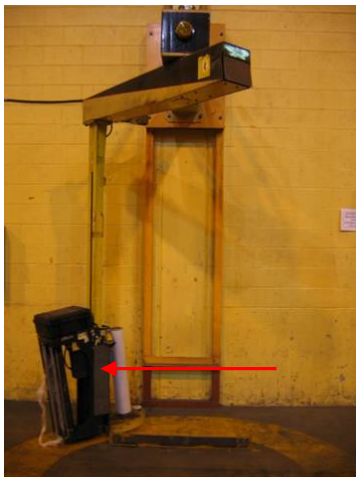
RFID Enhanced Stretch Wrap Machine
